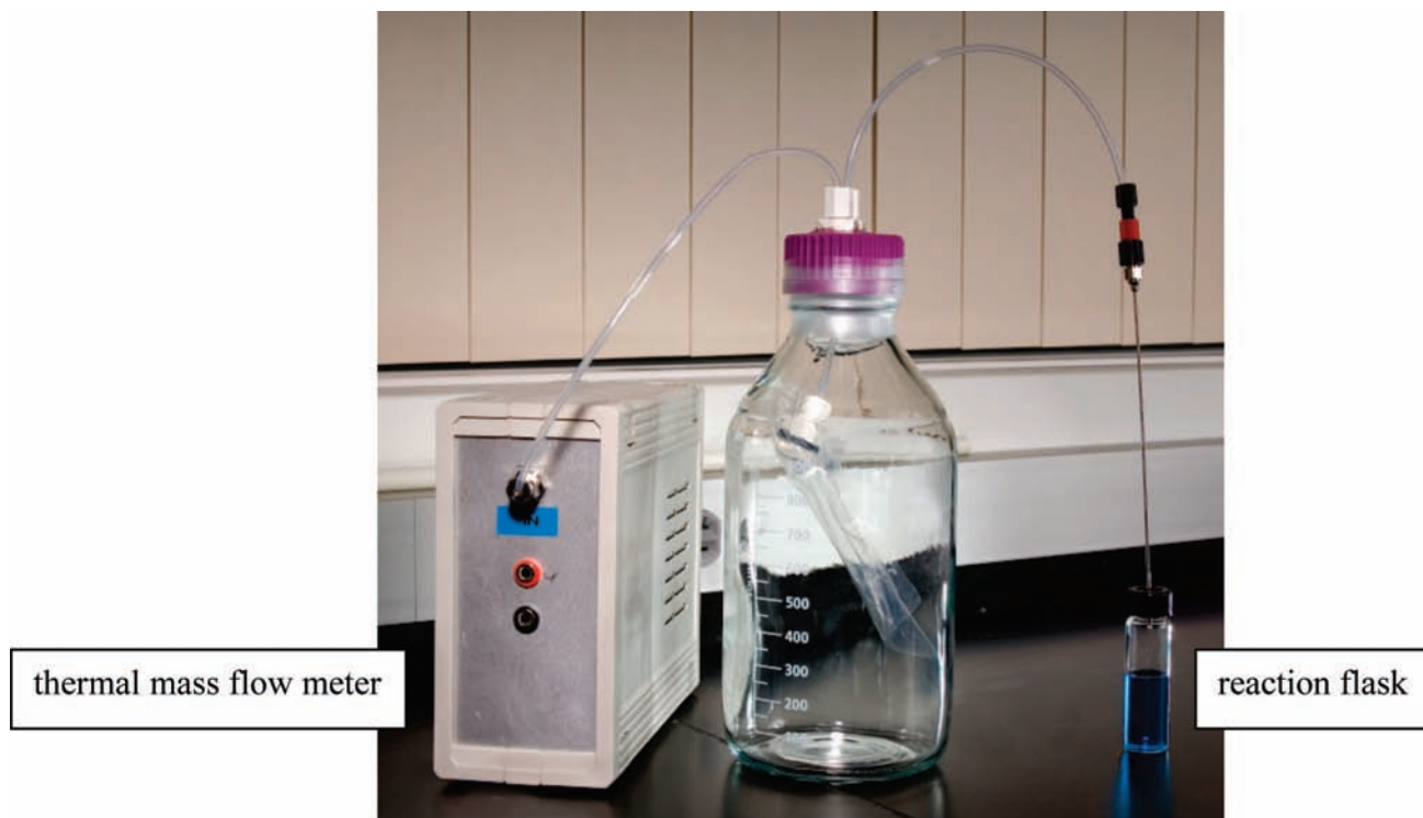
Figure 1. Picture of the bag in a bottle device that translates all gas flow to air flow. Off-gas from the reaction flask enters the bag causing it to expand which in turn forces air out of the bottle and through the thermal mass flow meter.
